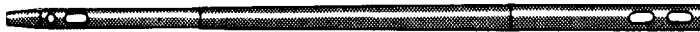
One-piece taper tie with slotted ends to be withdrawn for repeated use. Additional slot for two wall sizes.
